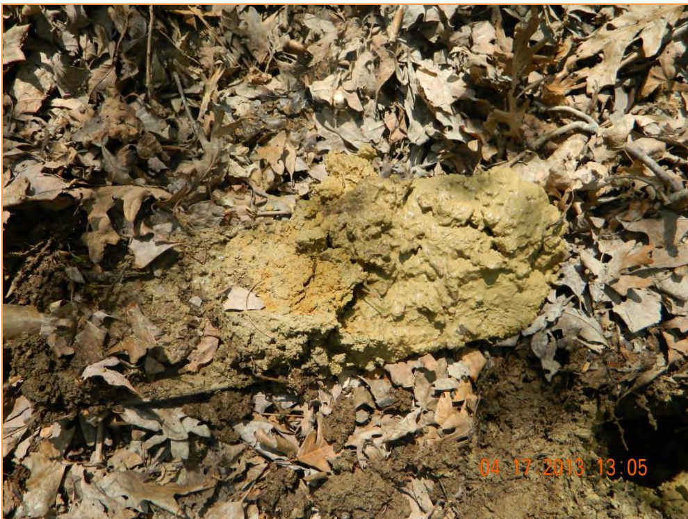
Photo 2 View of Silt Clay loam soil in WTL-1. Soil Matrix is 10YR 3/2 with mottles of 10YR 6/6
